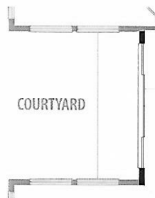
12ft Sliding Glass Doors at Courtyard
